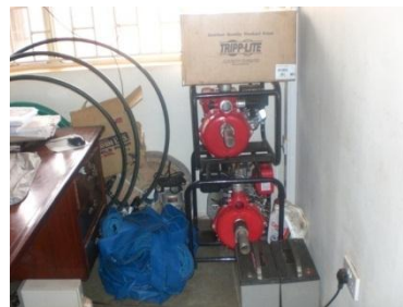
Petrol Driven pump can deliver up to 20,000 l/hr Irrigation Equipment ready for the field
