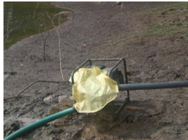
Petrol Driven pump can deliver up to 20,000 l/hr Irrigation Equipment ready for the field
